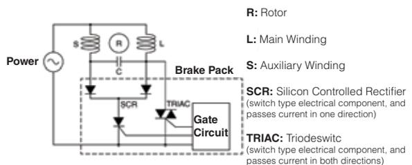
SCR is a circuit that flows the braking current. Only current from one direction flows.
