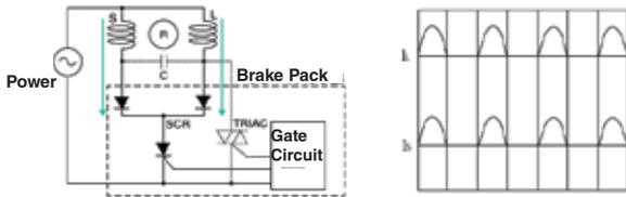
During instantaneous stop, a large braking current greater than the operating current flows. The braking current only flows for less than a second, so heat generation does not increase.
