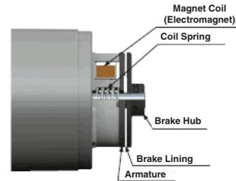
During motor operation, current flows through the magnet coil. The iron armature is attracted to the magnet coil which becomes an electromagnet when energized. As a result, the brake lining and the brake hub separate from each other, and the motor output shaft becomes free. While the motor is stopped, the coil spring pushes out the armature. As a result, the brake lining and the brake hub come into contact and hold the load.
